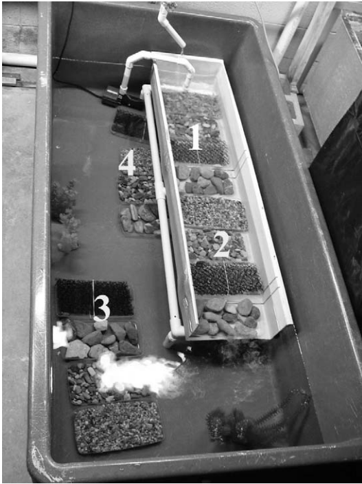
FIGURE 1.—Spawning tanks used to test the habitat and substrate spawning preferences of northern leatherside chub from March to September 2005. The four habitats were (1) upper riffle, (2) lower riffle, (3) uncovered pool, and (4) covered pool.
